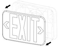
Drill or knock out appropriate knockouts on backplate to fit junction box mounting points.
