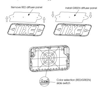
10. Remove proper "chevron" directional indicator(s) as required. When removing chevron(s), remove the color diffuser panel to allow easier access to the chevron(s). When color diffuser panel is removed, be sure to reinstall the color diffuser panel, securing with diffuser retention caps once chevron(s) has been removed.
